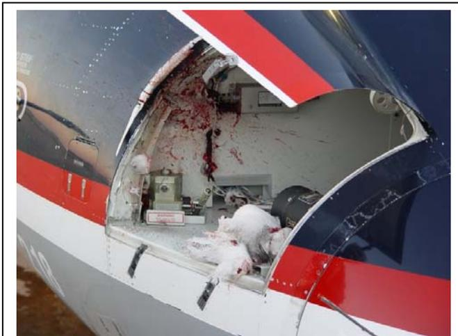
A CRJ 200 descending into a southern USA airport hit a flock of snow geese, 27 November 2007. Aircraft landed safely, but inspection revealed major damage to multiple components including 1 engine, nose, wing root and horizontal stabilizer.
