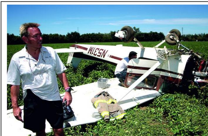
This Cessna 150 crash landed in a tomato field and was damaged beyond repair after a hawk shattered the windshield during approach to a California airport, 20 July 2007. Photo, Matthew Henderson.
