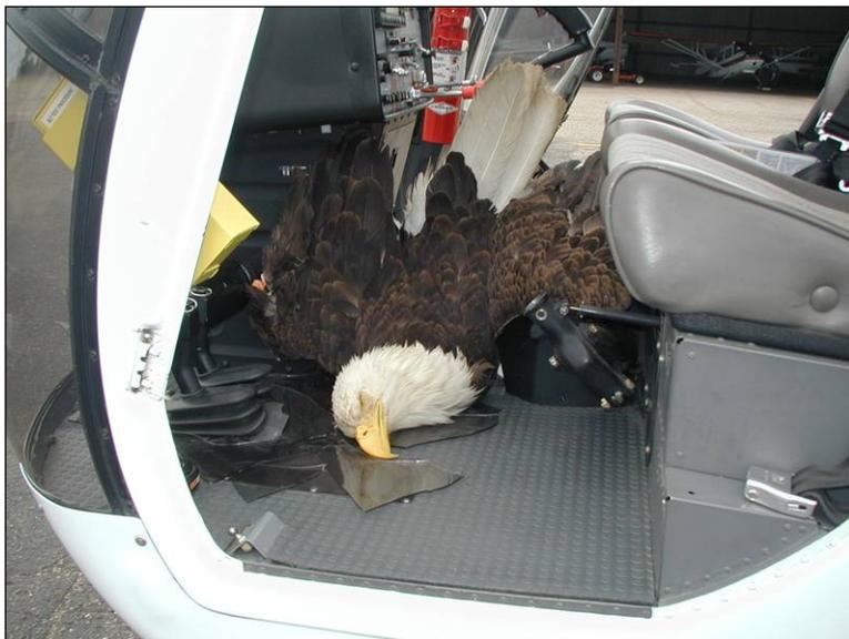
A bald eagle shattered the windshield of a Schweizer 300 helicopter at 2,000 feet AGL in Minnesota, 3 June 2007. The passenger was knocked unconscious and suffered cuts and bruises. Pilot landed the aircraft safely with the dead eagle at his feet. Photo, Chris Cooper, Hummingbird Helicopters.
