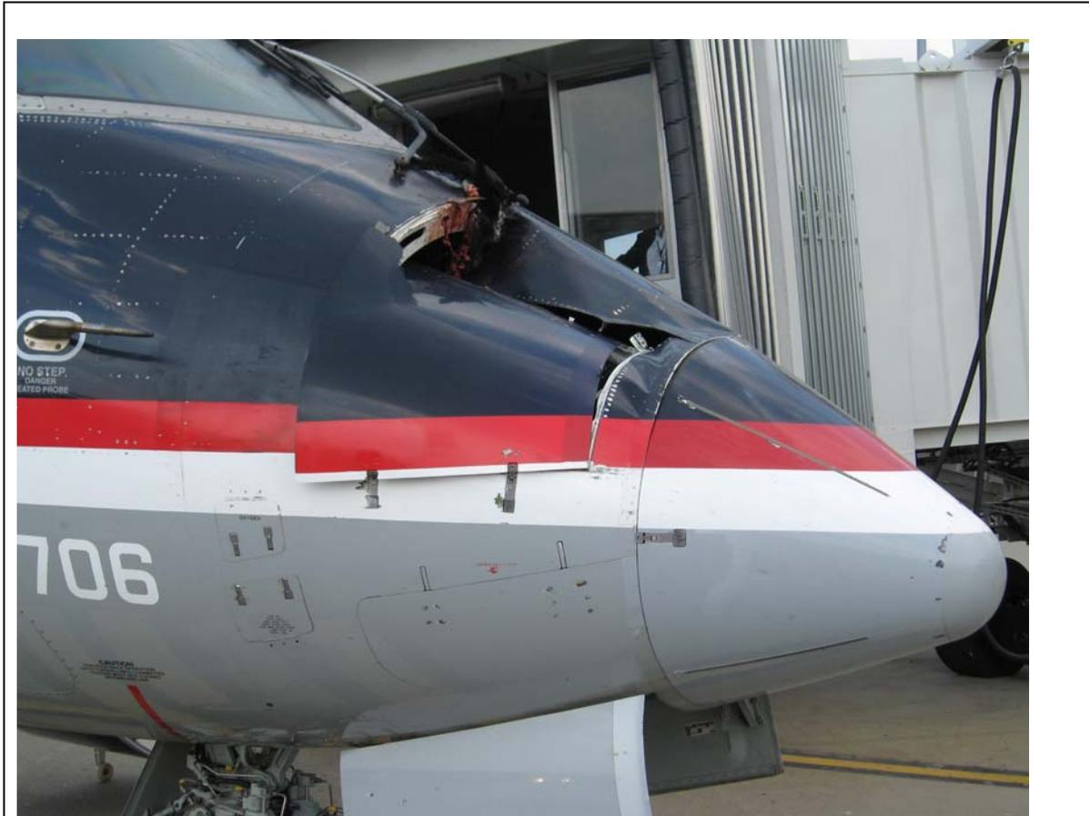
A CRJ-700 struck a black vulture on final approach to an airport in Kentucky on 28 August 2007. The strike caused substantial damage to nose cone. The black vulture population in USA increased at a mean annual rate of 2.6%, 1980-2006.
