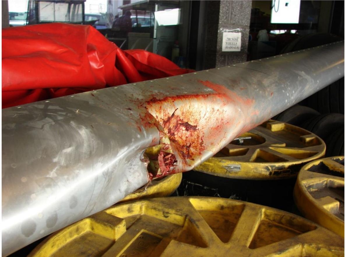
The leading edge of left wing of a B-737 hit a great blue heron on approach to an east coast USA airport, 7 November 2007. The pilot landed the aircraft uneventfully where it was taken out of service for repairs.
