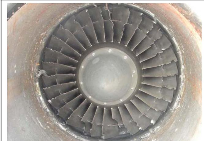
A Learjet 36 ingested a mallard into an engine during the takeoff run at a northern USA airport, 4 June 2007. Pilot aborted takeoff. Cost of repairs was >\$250,000.
